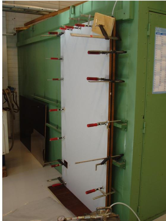
Figure 2. Vacuum filling of the PCM prototype. The PCM accumulator is between wooden plates during the filling.
