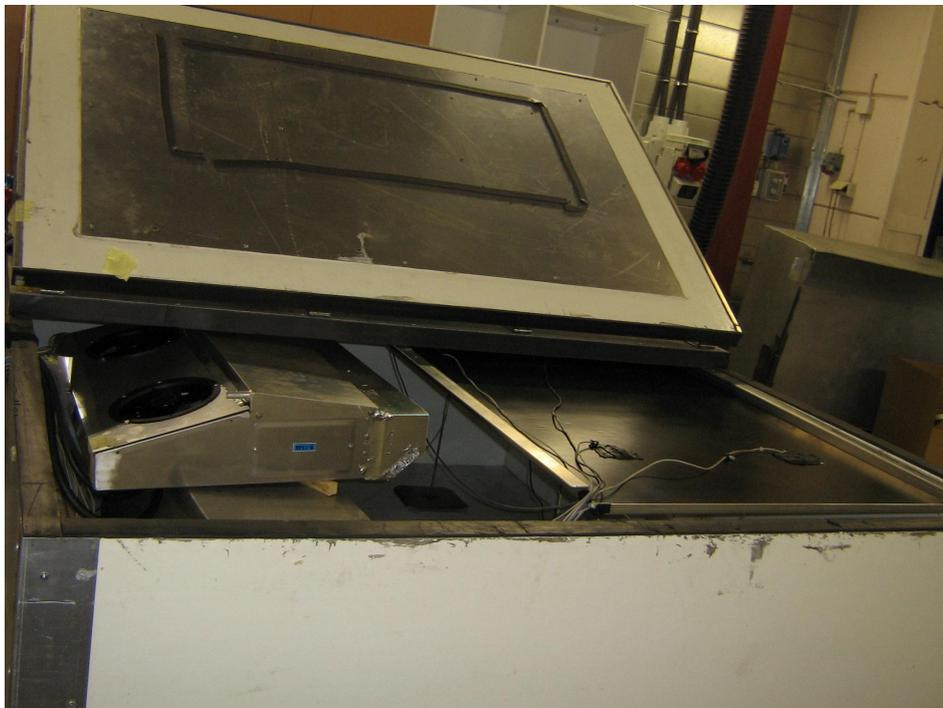
Figure 4. The PCM prototype module was assembled on the ceiling of the test box. The prototype is on the right and the refrigeration unit is on the left.
